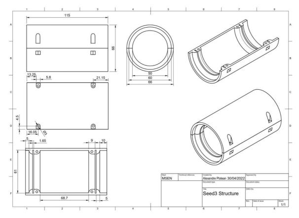
We opted to 3D print the CanSat (*Seed* 3) structure using PLA filament and in addition we also tried to print with bright colours filaments but we ultimately couldn't do it due to the lack of access to those colours.
